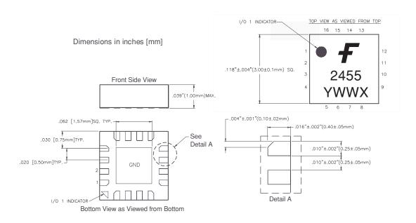
Note: Dimensions do not include protrusions or mold flash. These are not to exceed 0.006" (.155mm) on any side.
